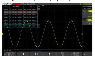
Playback the latest triggered events using the history function. Segmented memory collection will store trigger events into multiple (Up to 80,000) memory segments, each segment will store triggered waveforms and timestamp of each frame.
