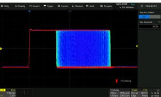
Segmented memory collection will store the waveform into multiple memory segments (up to 90,000) and each segment will store a triggered waveform together with the dead time information. The interval between segments can be as small as 2  $\mu$ s. All segments can be played backat an arbitrary frame rate using the History function.
