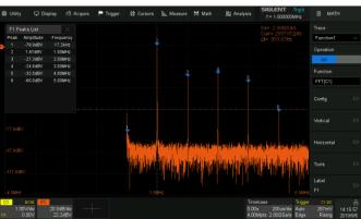
Hardware accelerated FFT up to 2 Mpts. This provides high frequency resolution with fast refresh rate. The FFT function also supports a variety of window functions so that it can adapt to different spectrum measurement needs. Three modes (Normal, Average and Max hold) can satisfy different requirements for observing the power spectrum. Auto peak detection and markers are supported.
