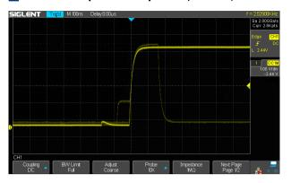
With a waveform capture rate of up to 500,000 wfm/s (sequence mode), the oscilloscope can easily capture the unusual or low-probability events
