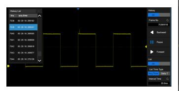
History function records up to 90,000 triggered waveforms (frames). This is done continuously in the background, so the history waveforms can be played back at any time to find and analyze past events. Serial decode, zoom and cursors measurements can be used.
