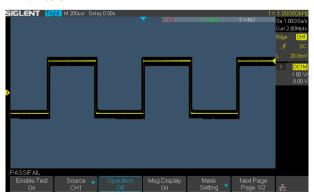
The SDS1000X-E utilizes a hardware-based Pass/Fail function, performing up to 40,000 Pass / Fail decisions each second. Easily generate user defined test templates provide trace mask comparison making it suitable for long-term signal monitoring or automated production line testing.
