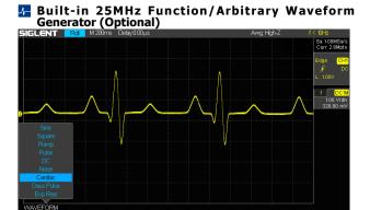
10 built-in waveforms plus 4 ARBs. The arbitrary waveforms can be accessed and edited by the EasyWave PC software
