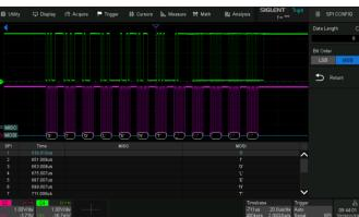
In addition to the decoder lanes correlated to the waveform, bus protocol information can be displayed in tabular form. I<sup>2</sup>C, SPI, UART, CAN, LIN, CAN FD, FlexRay, I<sup>2</sup>S and MIL-STD-1553B are supported.
