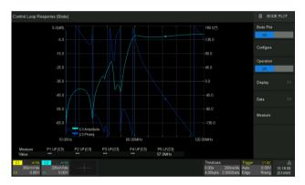
The SDS5000X can control the USB AWG module or a stand-alone SIGLENT SDG generator, to scan the amplitude and phase frequency response of the DUT, and display the data as a Bode Plot. This makes it possible to replace expensive network analyzer in some applications.
