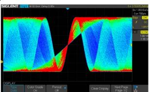
The color temperature display is similar to the intensity-graded trace function, but the trace occurrence is represented by different colors (color "temperature") as opposed to changes in the intensity of one color. Red colors represents the more frequent events, while blue is used to mark points that occur lest frequently.
