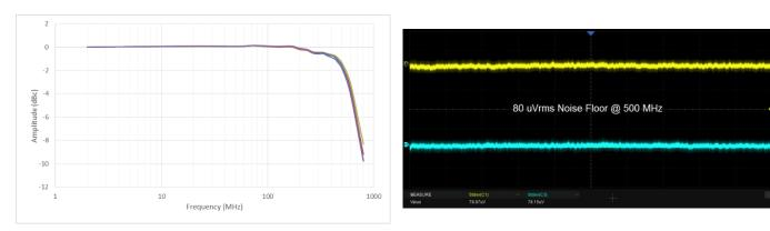
500 MHz bandwidth (at 2 GSa/s sample rate with 500 MHz Low noise floor: Only 80  $\mu$ V rms at 500 MHz bandwidth. bandwidth option).
