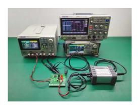
SDS1000X-E can control the USB AWG module or control an independent SIGLENT SDG instrument, scan a devices amplitude and phase frequency response, and display the data as a Bode Plot. There is also a Vari-level Mode for accurately measuring Power Supply Control Loop Response (PSRR). It can also show the result lists, and export the data to a USB disk.
