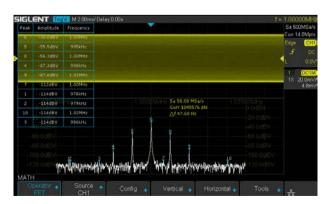
The new math co-processor enables FFT analysis of incoming signals using up to 1 M samples per waveform. This provides high frequency resolution with a fast refresh rate. The FFT function also supports a variety of window functions so that it can adapt to different spectrum measurement needs. Four-channel series support Peaks, Markers, a variety of numbers.
