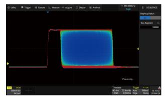
Segmented memory collection will store the waveform into multiple memory segments (up to 100,000) and each segment will store a triggered waveform as well the dead time information. The interval between segments can be as small as 2  $\mu s$ . All of the segments can be played back using the History function
