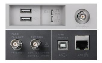
2 x USB Host, 1 x USB Device (USBTMC)1 x LAN (VXI-11/Telnet/Socket)1 x Auxiliary Output (Pass/Fail and Trigger Out)
