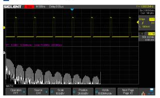
In addition to the traditional (+, -, X, /) operations, FFT, integration, differential, and square root operations are supported. The integration operation supports gating, which uses cursors to define the domain of integration
