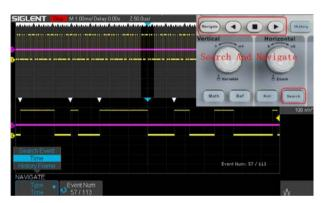
The SDS1000X-E can search events specified by the user in a frame. It can also navigate by time (delay position) and historical frames.
