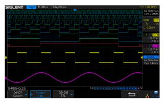
4 analog channels plus 16 digital channels enables users to acquire and trigger on the waveforms then analyze the pattern, simultaneously with one instrument.
