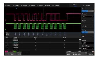
Display the decoded characters through the events list. Bus protocol information can be quickly and intuitively displayed in tabular form. I2C, SPI, UART, CAN, LIN, CAN FD, FlexRay, I2S and MIL-STD-1553B are supported
