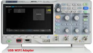
WiFi control of instrumentation can provide a convenient and safe method of configuring and collecting data. This new feature works with a SIGLENT approved WiFi adapter to provide wireless control and communications with SIGLENT 4 channel scopes. The adapter must be supplied by Siglent to ensure working.
