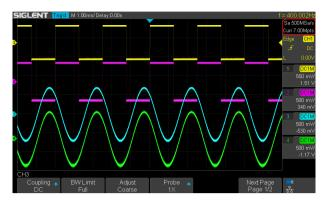
The four channel series has two 1 GSa/s ADC chips (channel 1 and 2 share one, channel 3 and 4 share another), so that each channel can achieve sample rates up to 500 MSa/s and work on bandwidths of 200 MHz when all channels are enabled.
