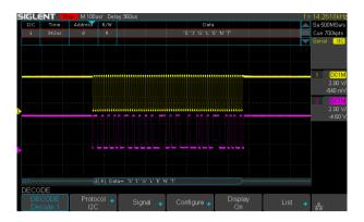
SDS1000X-E displays the decoding through the events list. Bus protocol information can be quickly and intuitively displayed in a tabular format.
