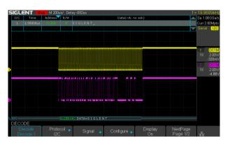
SDS2000X-E displays the decoding through the events list. Bus protocol information can be quickly and intuitively displayed in a tabular format.
