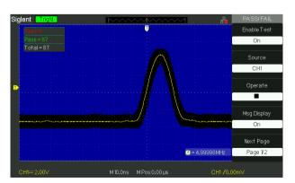
With easy to generate user-defined test templates, the SDS1000DL+/ CML+ compares the current measured trace to the template mask trace making it suitable for long-term signal monitoring or automated production line testing.
