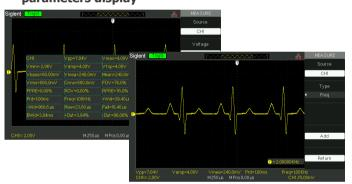
The SDS1000DL+/CML+ support voltage, time and delay measurement types, with a total of 32 different parameters. The user is able to select five measurements to display on the screen. All measurement parameters can also be displayed simultaneously.
