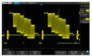
256-level intensity grading display on waveform
