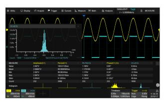
Statistics shows the current value, maximum value, minimum value, standard deviation and mean value of up to 5 parameters simultaneously. Histogram is available to show the probability distribution of a parameter. Trend is available to show the parameter value vs. time.
